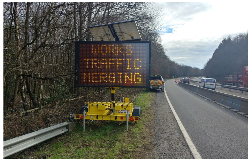
Mobile VMS on the A21 Kippington (Chevron, Costain) displaying Work's Egress activation message to passing motorists upstream from Site exit
